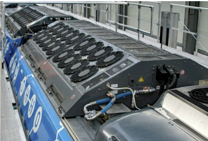
Roof Mounted Fuel Cell
